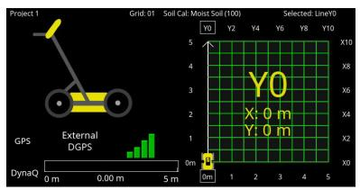
The LMX150<sup>TM</sup> FINDAR\* GPR guides you through the setup with pre-selected grid sizes. Stop lines early, or skip lines.
