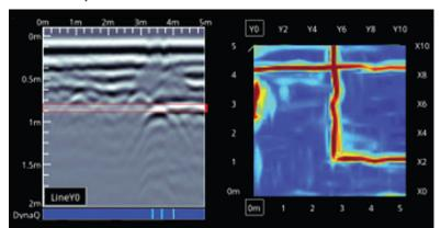
Process grid data into depth slices and move down through your data to visualize targets at different depths.
