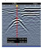
No complex settings - Just press start and push the cart Use hyperbola - fitting to ensure accurate depth measurements and backup over the target to display its location and depth.
