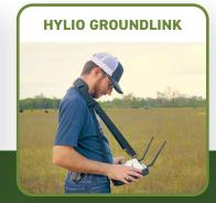
Hylio proprietary, NDAA compliant ground station. An integrated Window tablet and RC controller which allows you to seamlessly switch autonomous and manual controls for one or multiple drones.
