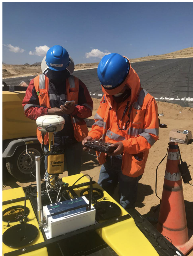
Different Setup Configurations in Hypack Survey for Bathymetries with the HyDrone-ANP
