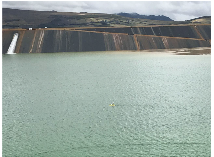
Autonomous Tailings Pond Bathymetry Using a HyDrone-ASV Equipped with a HydroLite Echosounder
