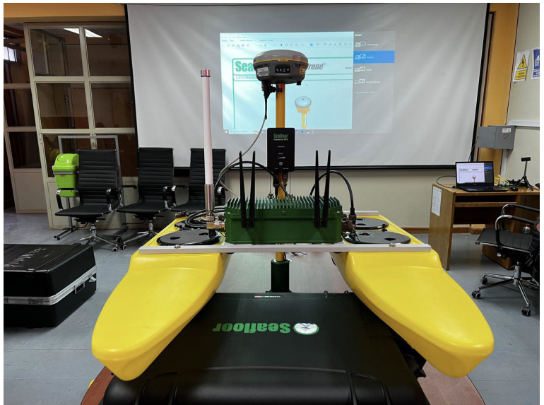
HyDrone-ANP with HydroLite Plus Dual and Trimble R8s - Setup for Training
