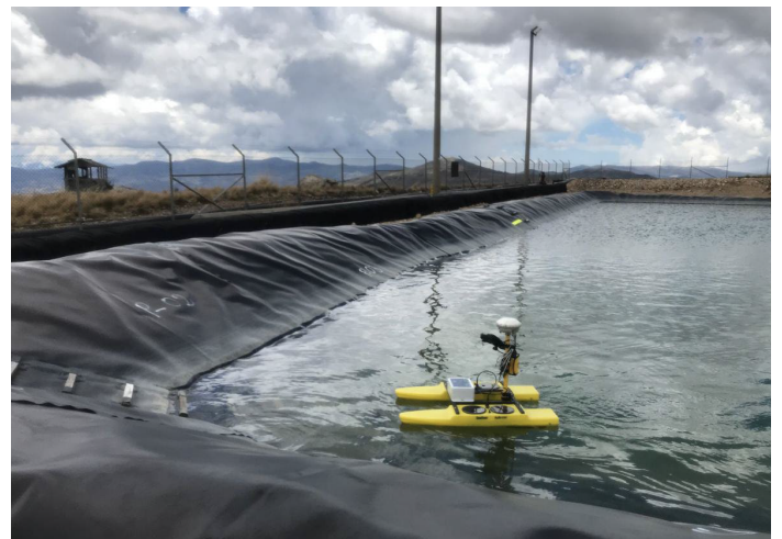
Conducting a Bathymetric Survey to Verify the Volume of a Process Water Pond
