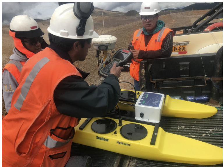
Setting up the HyDrone-ASV with HydroLite to collect bathymetric data with Trimble Access
